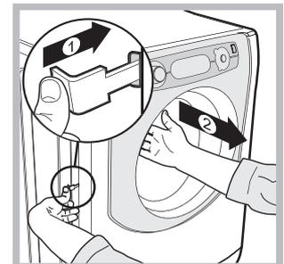
4. Press down on the key while pulling the handle outwards to open the door.
