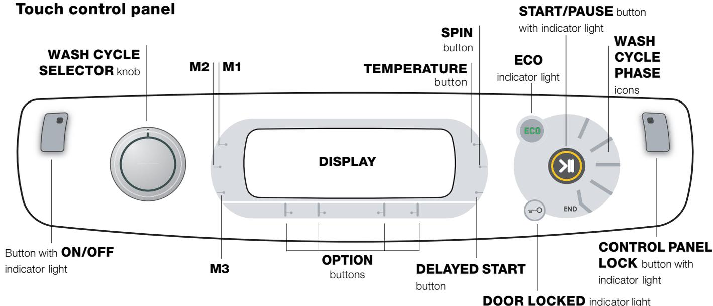
Button with **ON/OFF** indicator light: press this briefly to switch the machine on or off. The green indicator light indicates that the machine is switched on. To switch off the washing machine during the wash cycle, press and hold the button for approximately 3 seconds; if the button is pressed briefly or accidentally the machine will not switch off. If the machine is switched off during a wash cycle, this wash cycle will be cancelled.
